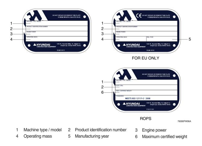
\* The product identification number (machine serial number) assigned to this particular machine and should be used when requesting information or ordering service parts for this machine from your authorized HYUNDAI dealer. The product identification number is also stamped on the frame.
